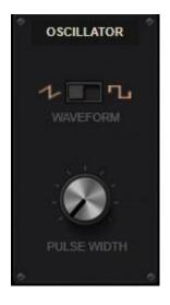
WAVEFORM: Toggles between Saw (Sawtooth) and Pulse (Square) oscillator shapes.
