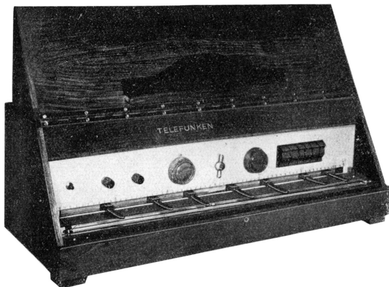
FIGURE 23. The Telefunken-Trautonium, also known as the Volkstrautionium. Source: Peter Lertes, Elektrische Musik (Dresden: Theodor Steinkopff, 1933), 184.
