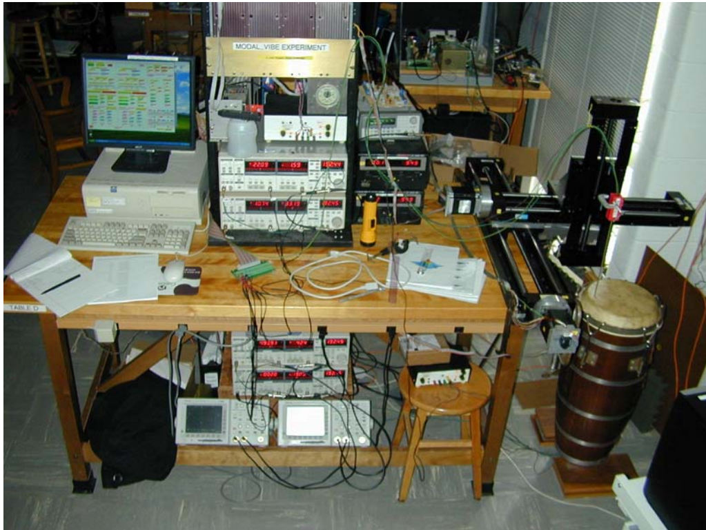
Figure 30: The setup is shown in the lab. The drum to the right is the Brazilian drum that we have measured on. The computer is used for collecting data and the four lock-in amplifiers are shown in the middle of the picture two above and two below the
