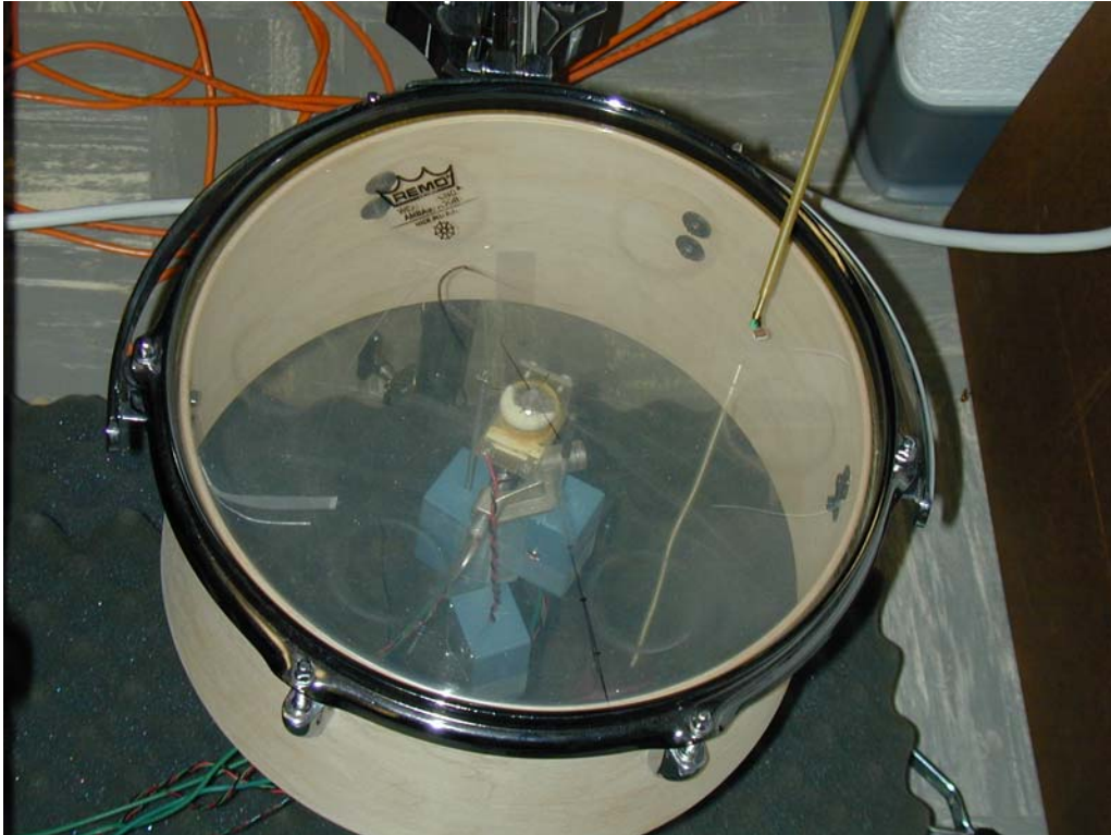
Figure 32: The figure show a Tom drum used in a previous experiment. Through the membrane one can see the two microphones and the electromagnet that is placed below the membrane. The stick coming down from above is holding the two microphones above the membrane.
