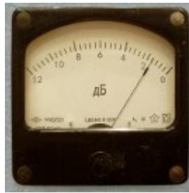
Pic 8. Indicator scale switched to 12 dB
